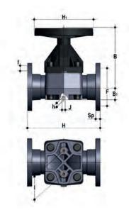
**VMOAC**Diaphragm valve with flanged monolithic body, drilled ANSI B16.5 cl.150 #FF
