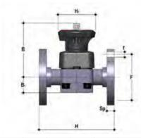
DIALOCK® diaphragm valve with flanged monolithic body, drilled PN10/16. Face to face according to EN 558-1
