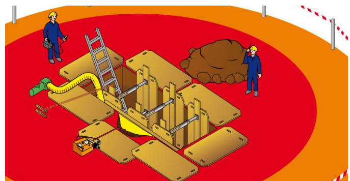
Multiple safe zones in a trench
